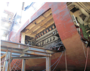
WHEELER in Drydock, engine and ship prepared for moving in one piece
