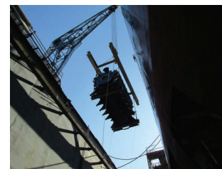
Main Engine Clearing The Drydock
